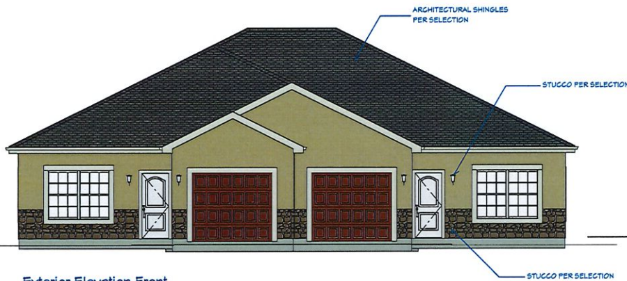
Exterior Elevation Front
